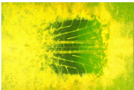
Full Tread Depth at 55 mph in Wet Conditions
