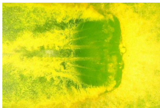
Half Tread Depth at 55 mph in Wet Conditions
